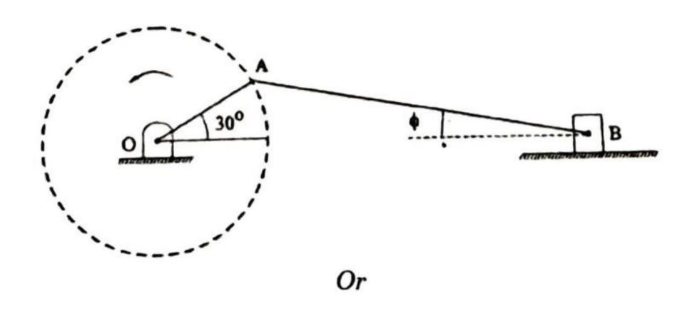
(b) In the reciprocating engine mechanism as shown in figure, the crank OA rotates at a uniform speed of 300 r.p.m. The lengths of crank and connecting rod are 12 cm. and 50 cm. respectively. Find (i) The angular velocity of the connecting rod AB; and (ii) The velocity of piston when the crank makes an angle of 30° with horizontal. Use instantaneous centre approach.
