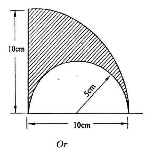
(b) Calculate the moment of inertia of the shaded region as shown in figure with respect to the centroidal axes.
